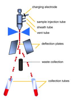
Figure 6-2 Sorting components on the FACSVantage SE
