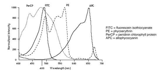
Figure 3-3 Absorption spectra of four common fluorochromes
