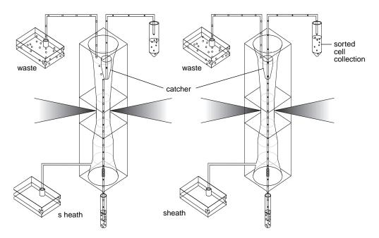
Figure 6-1 (Left) catcher tube in sheath stream; (right) catcher tube in sample stream
