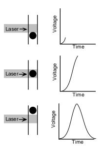
Figure 4-5 Creation of a voltage pulse
