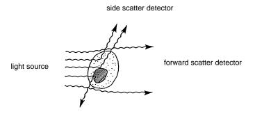
Figure 3-1 Light-scattering properties of a cell
