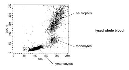
Figure 3-2 Cell subpopulations based on FSC vs SSC
